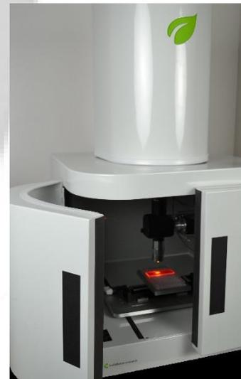
more intense non-chlorophyll wavelength region. With this filter in place, more laser light could be delivered to the sample without saturating the CCD at these wavelengths [4]. By delivering more laser light, we increased our sensitivity for the earliest signs of chlorophyll within the seed. This collection mode up-weighted and concentrated the imaging on the chlorophyll spectral region (Figure 1).
